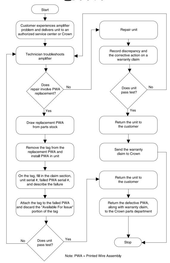
Figure 1.2 Service Procedure Flow Chart
