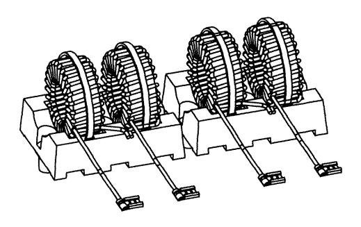
View of Inductor Pair, CPN H43507-5, for Output Assembly CPN 101554
