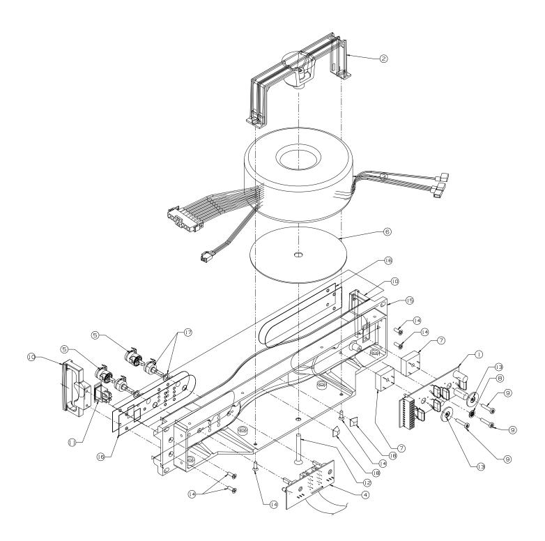
Figure 7.2 Front Panel Assembly Exploded View
