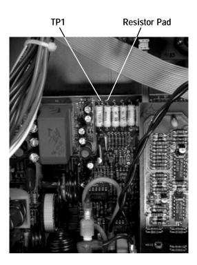
Figure 5.1 Discharge Test Point
