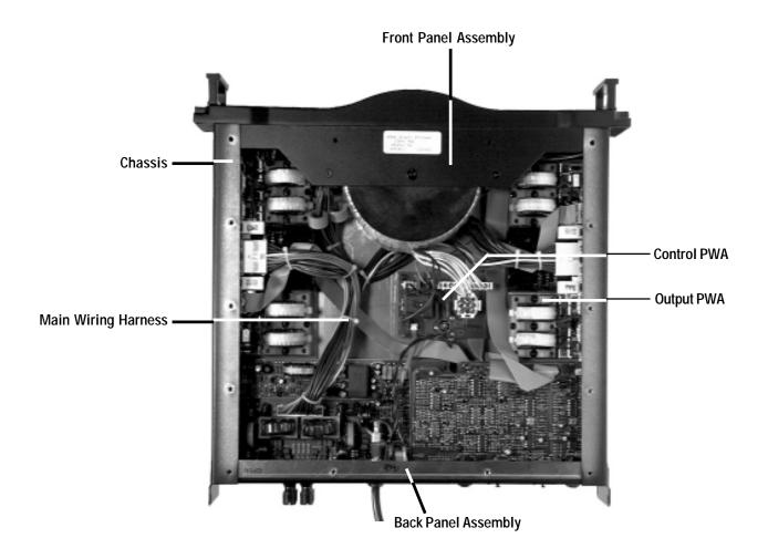
Figure 7.1 View of Main Chassis from Bottom
