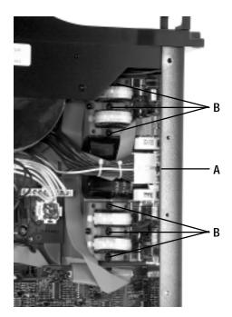
Figure 5.3 Output PWA Screws
