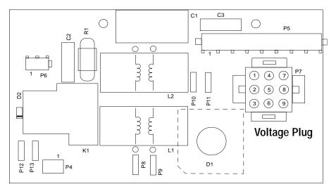
Figure 4.2 Control PWA with Voltage Plug
