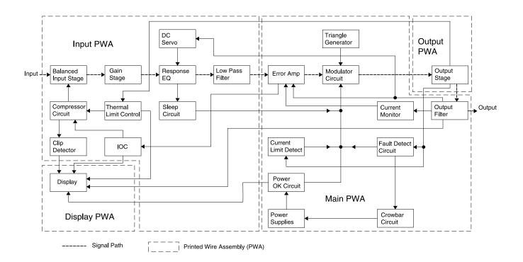
Figure 3.1 Amplifier Block Diagram
