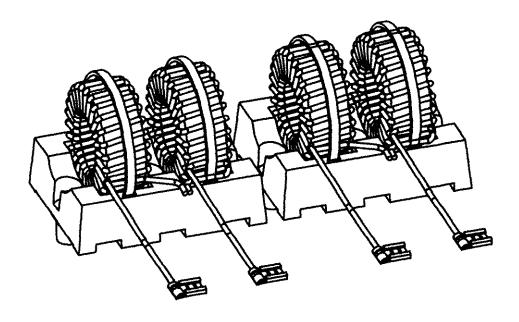
View of Inductor Pair, CPN H43507-5, for Output Assembly CPN 102175-2
